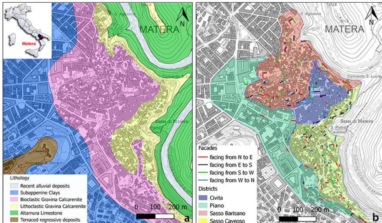
Figure 1 – (a) Schematic lithological map of Matera; (b) Map of the Matera Sassi. Polygons of different colors highlight the Sassi sub-districts. The analyzed façades are reported respect to the exposition.
