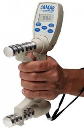
Figure 7 – Jamar Plus+ handgrip is a digital dynamometer used to determine the grip strength (weakness) at both hands, left and right. For each hand two tests are made and the measurements that appear on the display of the dynamometer are collected: grip strength (kg), average between the two measures made for each hand (AVG, kg), standard deviations (SD, kg) and coefficient of variation (CV, kg).
