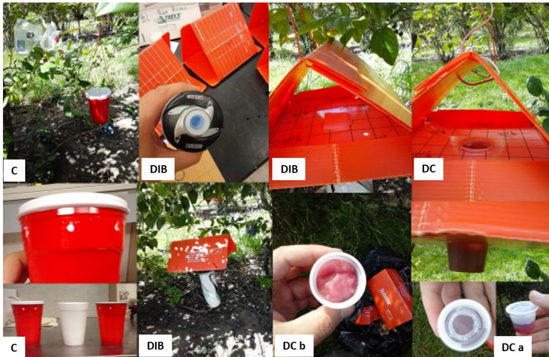
Picture A 3.1. Trap types: C- Red cup with a white lid; DIB- Delta trap with an insulated bottle; DC- Delta trap with a cup without a lid, with two cotton balls.
