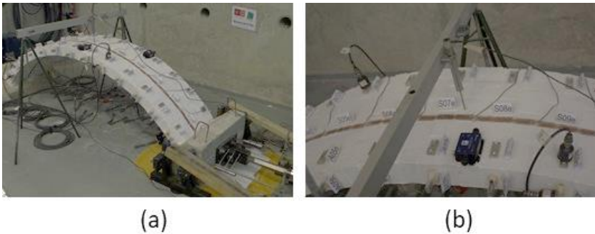
Figure 6.14. Arch test: a) view of the test apparatus; b) vertical LVDT
