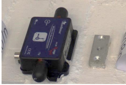
Figure 6.17. BeanDevice® AX-3D XRange wireless vibrations sensor
