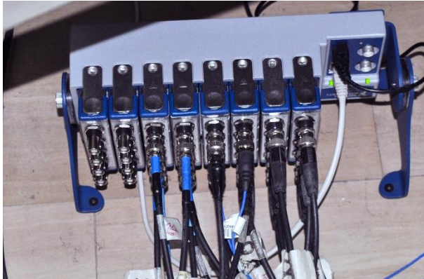
Figure 5.21. Modular chassis and modules for the acquisition system.
