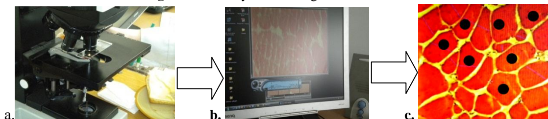
Figure 14.2. Way of counting the number of fibres
