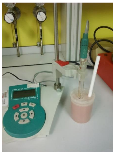
Figure 6.33. pH determination in an homogeneizate chicken patties sample
