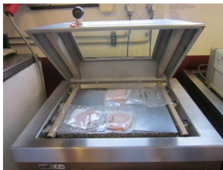
Figure 6.21. Patties packed in different vacuum high oxygen barrier bag
