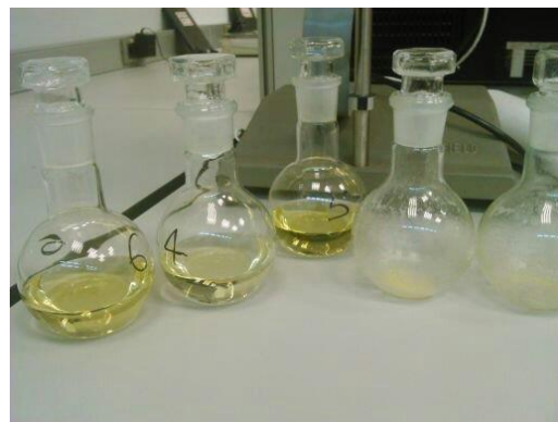
Figure 6.2 Fat extraction from chicken meat samples, before and after rotavapor
