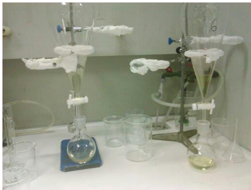
Figure 6.1. Fat extraction from chicken meat samples
