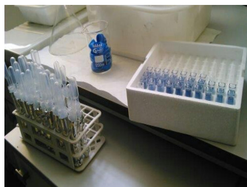
Figure 6.30. Samples after 1h of Folin–Ciocalteu reaction in dark
