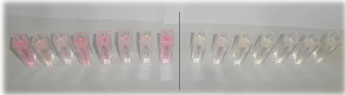
Figure 6.4. Cuvette of Vitamin E group (left side) and Control group (right side) during the spectrophotometer reading (96h). It is possible to observe the different coloration ( personal photo )
