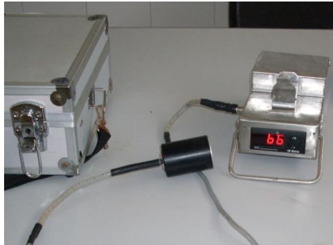
Figure 6.3. Artificial vagina with temperature maintaining
