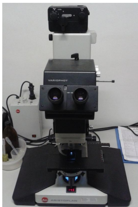
Figure 5.6. Phase-contrast microscope (Leica Aristoplan; Leitz Wetzlar, Heidelberg, Germany)
