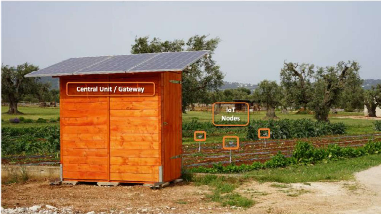
Figure 3.1. Central unit of the solar fertigation system connected with the internet of things (IoT) with the help of wireless sensory networks (WSN) at crop field conditions.
