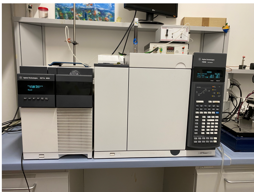
Fig. 13 - GC-MS Agilent 5977A mass selective detector (MSD).
