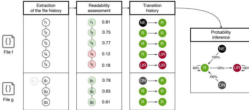
Figure 7.2: The process we used to compute the transition probability of a project.
