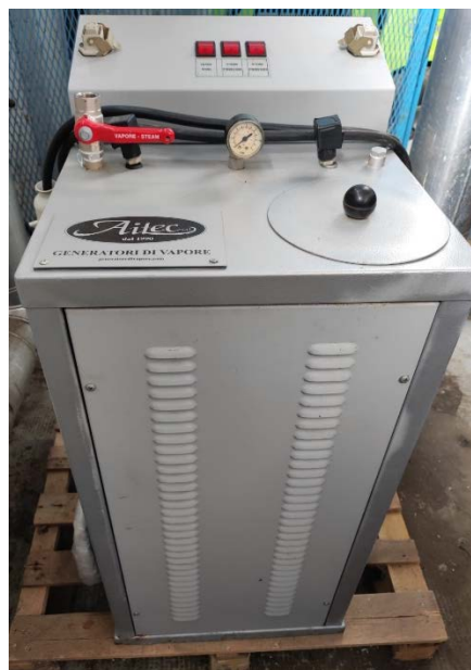
Figure 8.24 - New steam electrical boiler for next experimental activities, using an oxy-steam gasification approach.
