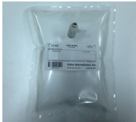
Figure 6.45 - Syngas sampling bag.
