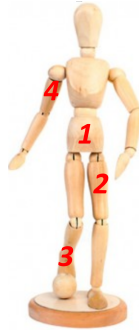
Figure 2.2: Wearable devices scheme of positioning: (1) waist, (2) left thigh, (3) right ankle and (4) right arm.
