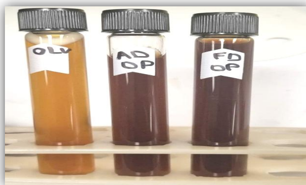
Fig. 17_ Methanol-extracted compounds derived from olive oil by-products (OIBP) using the ultrasound bath extraction technique (UB-EX)
