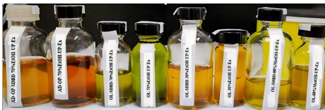
Fig. 39 _ Color difference in extracts prepared b Ultrasonic probe extraction with and without Surface Dielectric Barrier Discharge (SDBD) Pretreatment
