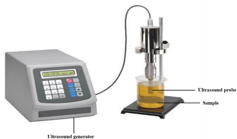
Fig.5_ Working principle of ultrasound-assisted extraction (UAE) (Huezo et al. , 2019)
