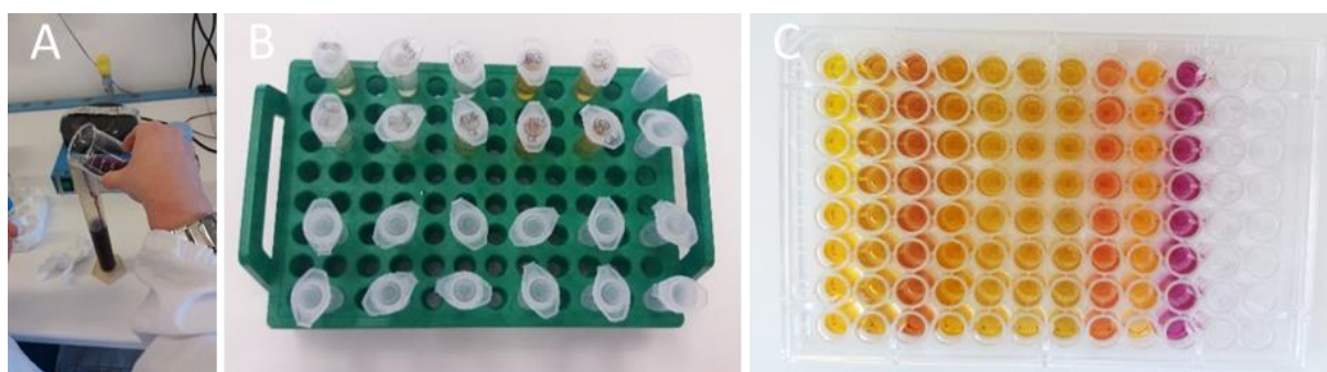
Figure 8 a) Reagent solution preparation; b) Reagent solution and culture filtrate mix; c) 96-well microtitration plates setting
